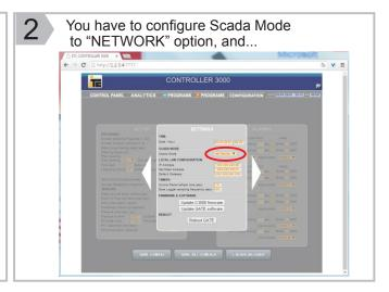
in LOCAL LAN CONFIGURATION you have to put a IP Address, NetMask and Default Gateway, according to the Local Network where you want to connect the GATE
