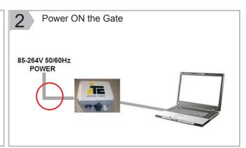
Configure Ethernet adapter in your PC with following configuration: IP Address: 10.1.1.1
