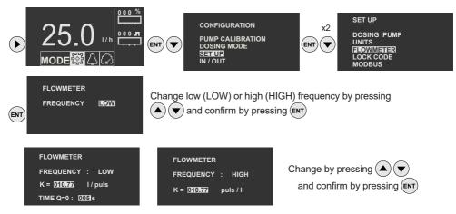
TIME Q=0, Time interval (seconds) between two pulses to consider zero flow.
