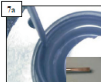
7a Insert the o'ring inside the groove pressing it with a screwdriver
