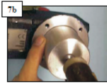
7b You can also introduce the o'ring using a tool as showed in the picture
